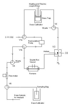
Figure 1: Synthesis apparatus schematic.
